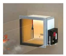
A fire breaks out and the temperature reaches 72°C: the fusible link melts and the damper blade closes.
