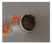
Two blocking hooks lock the blade in the closed position, and the intumescent material expands, providing a perfect seal to stop flames and smoke.
