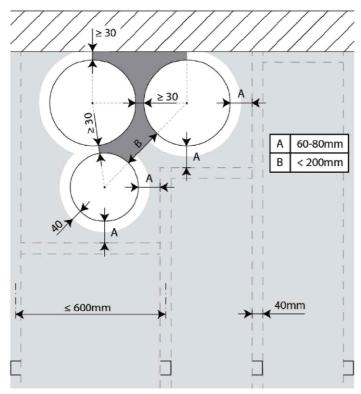
Mounting in a rigid wall at 0 distance
