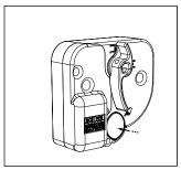
1. Unlock the existing mechanism by pressing the unlocking button.
