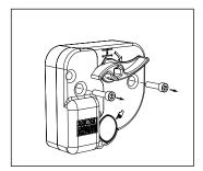
2.Loosen up the 2 fixing screws with the enclosed hex key and dismantle the existing mechanism.
