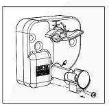
6. Mount the fusible link and tighten up with the screw.
