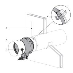
A. CRE60 damper installed remotely from the supporting construction.
