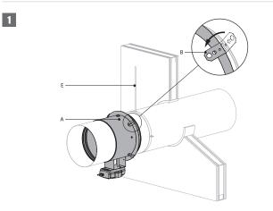
A. CRE60 damper installed remotely from the supporting construction.
