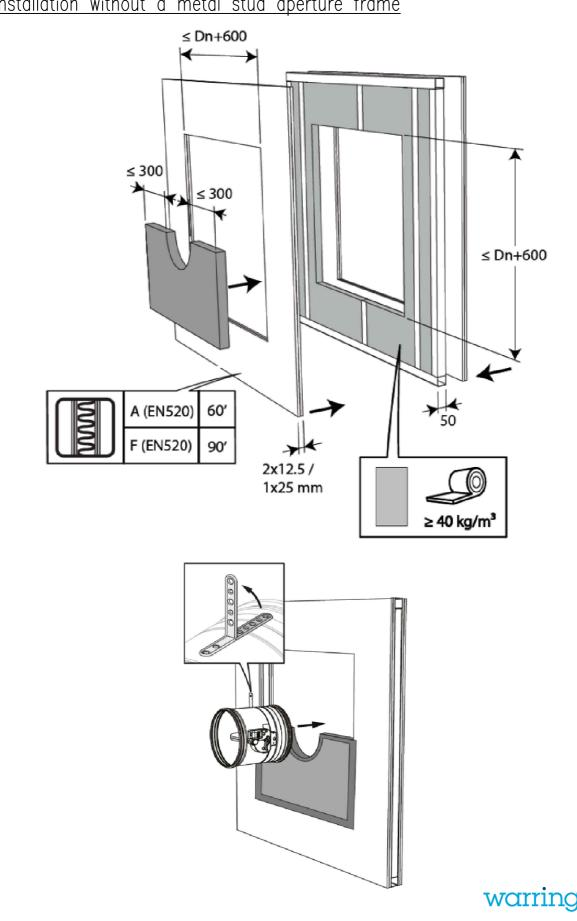
Installation without a metal stud aperture frame
