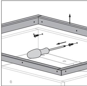
1. Remove the screws and take off the PS flange.
