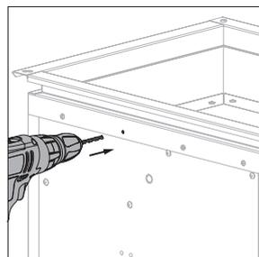
6. Drill these central holes through to a diameter of 5 mm
