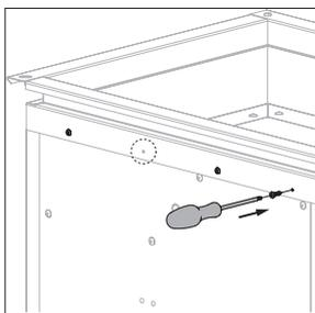
5. Fasten the flange with delivered chipboard 40 x 1.5mm screws except one of the central holes at each side of the flange.
