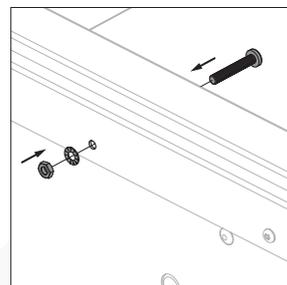
7. Fasten the delivered M5 bolts (head of the screw on the inside of the damper).
