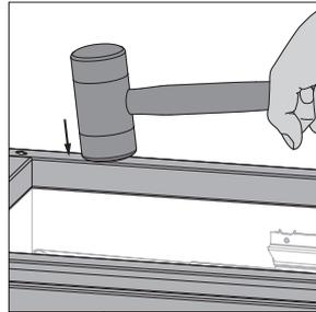
2. Place the connection flange over the casing and gently tap with a hammer.
